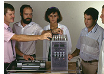
This "PCR" instrument was developed in the lab of Prof. Paul van Helden in 1989. It was made entirely in-house and is based on 4 supermarket hairdryers. The "developers" are shown, from left to right: Prof. Tommie Victor, Prof. Paul van Helden, Rene du Toit (Technologist), Frank Peiser (electronics), Cor Wijtenburg, (metal working).
