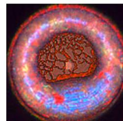
*Optical microphotographs of several attempts to deposit colloidal crystals on photonic fibers resulting in a donut and a bean, illustrating the beautiful colors of opals so formed. The diameter of the donut and the thickness of the bean are approximately 125 microns (300X magnification).*
